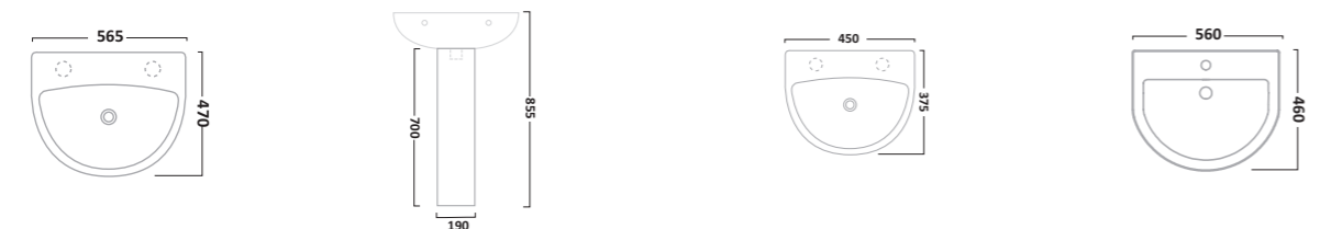
565mm Ceramic Basin 1 Tap Hole SB100S, 2 Tap Holes DB100S Pedestal PE100S 450mm Ceramic Basin 1 Tap Hole SB145S, 2 Tap Holes DB145S 560mm Semi-Countertop Basin 1 Tap Hole M3SCBAS
