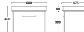
600mm Wall Mounted Unit Gloss White CM600WW Gloss Light Grey CM600WG Gloss Clay CM600WC
